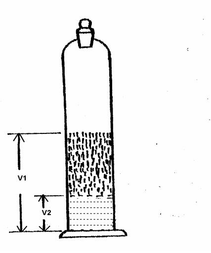
Figure A.1 — Measurement of foam
