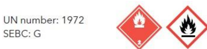
Figure 7: Hazard Pictogram LNG (Source Marine HNS Response Manual Multi-regional Bonn Agreement, HELCOM, REMPEC, pg 141)
