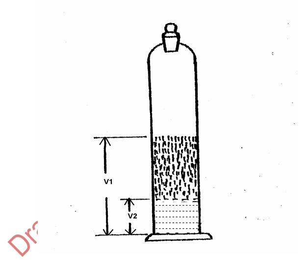
Figure A.1 — Measurement of foam
